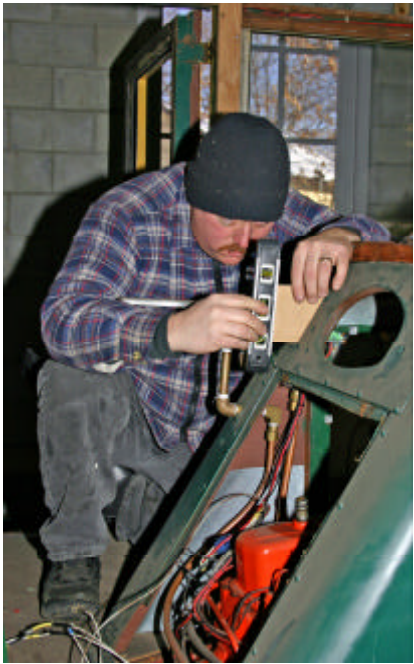
Bill Voorvaart works on the throttle mechanism for the Maine Central Rail bus. – (Robert A. LaMay photo)
