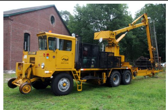
We thank the P&W Railroad for sending their Hi-Rail Bridge Crane Truck to Railroad Day. (Robert A. LaMay Photo)
