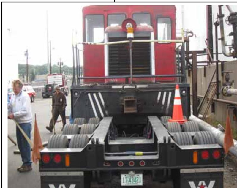
This view shows the 45 ton locomotive after it was loaded onto Vito's Trucking Co. trailer at New Haven, CT. Once it arrived at Willimantic it was offloaded onto the tracks. (Francis Saunders Photo)
