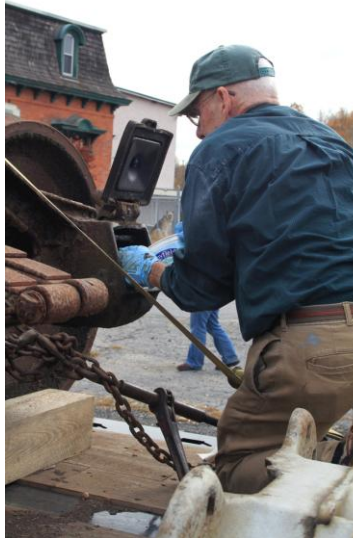
Bob Hassett pours lubricant in the journal box so when the caboose is put on the trucks it will move ever so smoothly on the rails to Columbia Jct. (Robert A. LaMay Photo)
