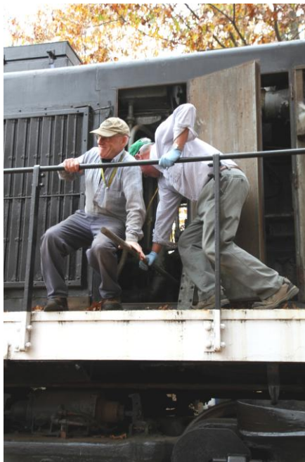
Here Bob Hassett and Cliff Lund push down on the bar which helps turn the engine's crankshaft. (Bob LaMay Photo)
