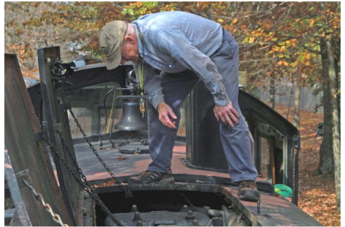
After opening the access panels above the engine Bob Hassett takes a closer look at the compression valves on the engine. (Robert A. LaMay Photo)
