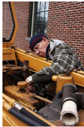
Paul Shamonis II install a carburetor into the IH back-hoe just outside the roundhouse. (Robert A. LaMay Photo)
