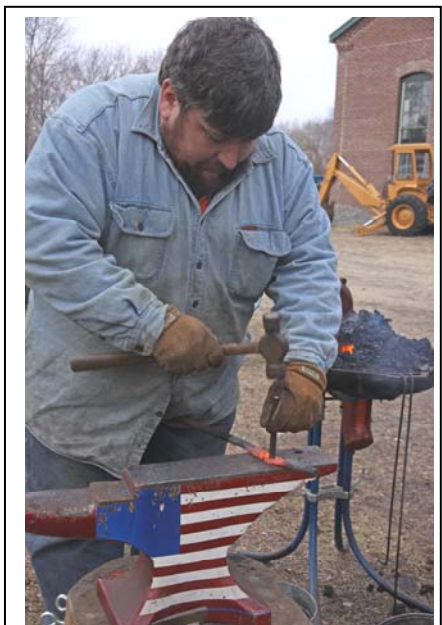
Rich Cizik applies his blacksmith skills while making a couple handles for the Gallows Signal. These will assist in raising and lowering the signal boards. (Robert A. LaMay Photo)
