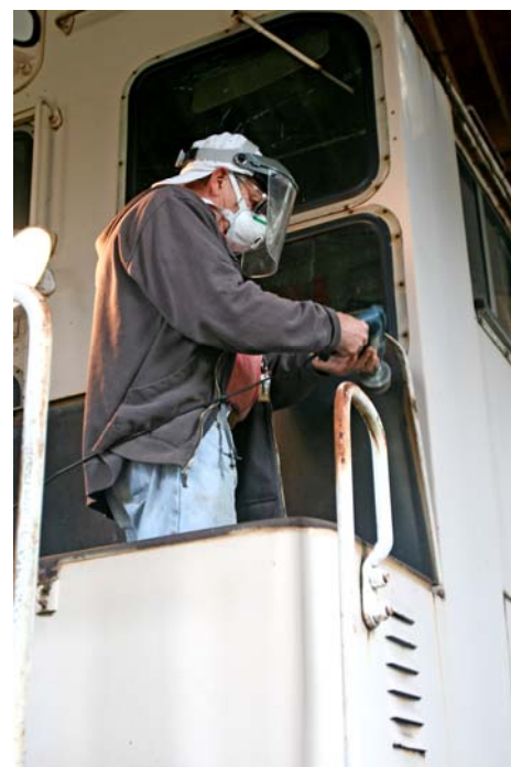
Rolf Johnson cleans up the battery box on the SW8 before installation of its batteries. (Robert A. LaMay Photo)
