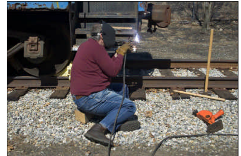
Steve Melady welds the steps back on to the ex-NH caboose recently moved to the museum. R.A. LaMay photo
