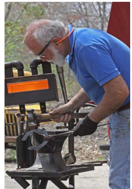
Barry Hulse a Ferrier from Pomfret Center, CT shows how horse shoes are forged on an anvil. (Robert A. LaMay Photo)
