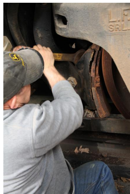
Jim Poor works on replacing the brake shoes on the SW8 locomotive inside the roundhouse. (Robert A. LaMay Photo)
