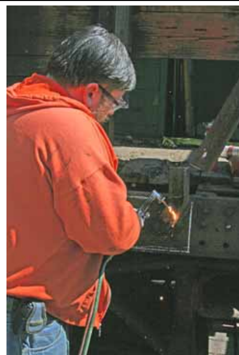
Rich Cizik uses a little heat to remove some rusted areas of number 4052 during its restoration. (Robert A. LaMay Photo)
