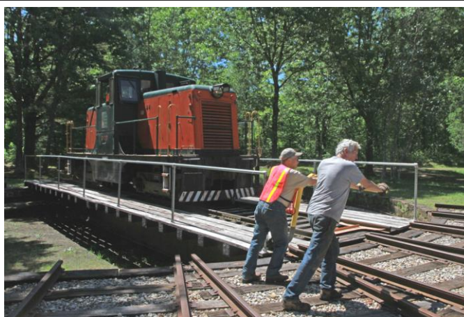
Duke York on left and Art Hall Jr. turn the Armstrong turntable with the 44 ton locomotive. (R. A. LaMay Photo)
