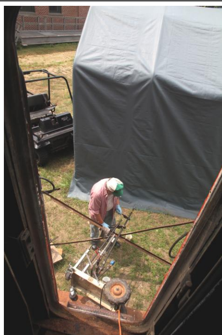
This view from inside the FL9 shows Rolf Johnson working on the pre-luber which will be used for starting locomotives that have been idle for some time. (Robert A. LaMay Photo)
