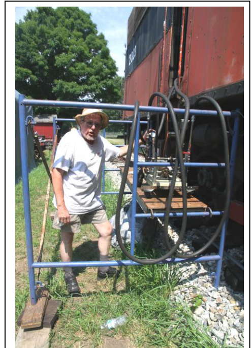
Master Inventor at work – Rolf Johnson poses during the pre-lube of the FL9, which hopefully will make it easier to start. (Robert A. LaMay)
