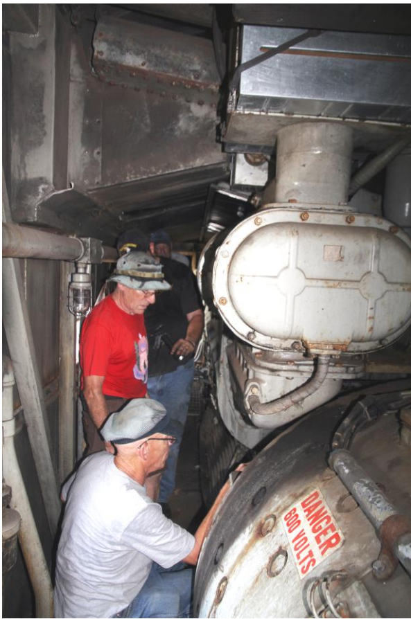
Paul Shamonis II, Jim Poor, Bob Hassett, and Gerry Roy work during the pre-lube of the FL9 to turn the prime-mover over. (Robert A. LaMay Photo)
