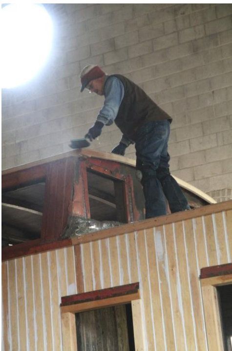
Duke York works on the cupola section of the Central Vermont Caboose #4052 during its complete restoration. (RA LaMay Photo)
