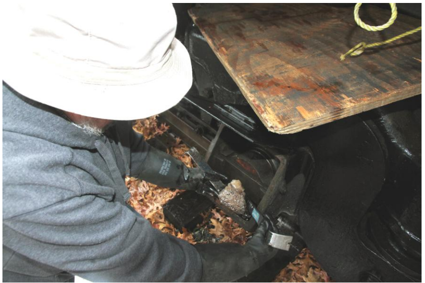
One of the hazards of winter is the ice that forms inside the journal boxes of the Central Vermont Alco S4 locomotive. Shown here Rolf Johnson removes a chunk of ice from the journal box. (Robert A. LaMay Photo)
