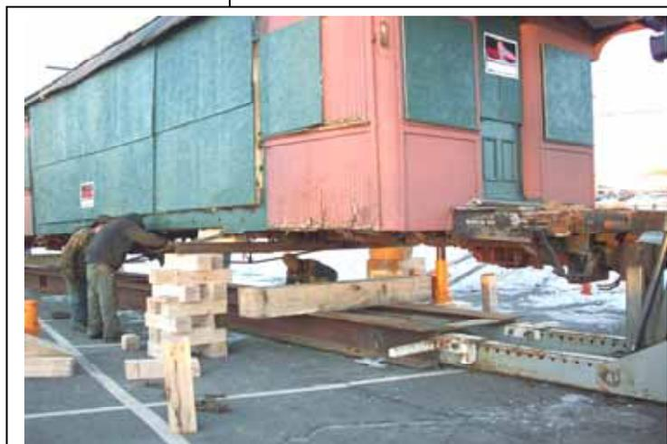
With both wheel sets (trucks) removed, the lowering begins. Note the trailer underneath the car. Plan is to lower the car onto this trailer, connect the wheels and harness assemblies, and off it goes.
