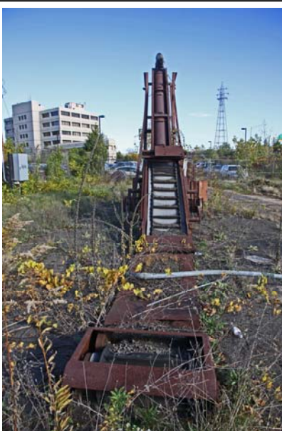
This is the view facing Hartford of the un-loader/auger prior to its dismantling. In the foreground is where the material was loaded before it traveled along the conveyor and into trucks. (Robert A. LaMay Photo)
