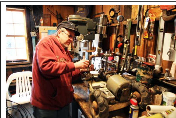
Rolf Johnson is in the section-house working on a new item to be used at the museum. It's called a motorized pre-lube. Basically what it does is pushes oil through the engine of a locomotive which makes the starting much smoother and less stressful on the engine parts. (R.A. LaMay Photo)
