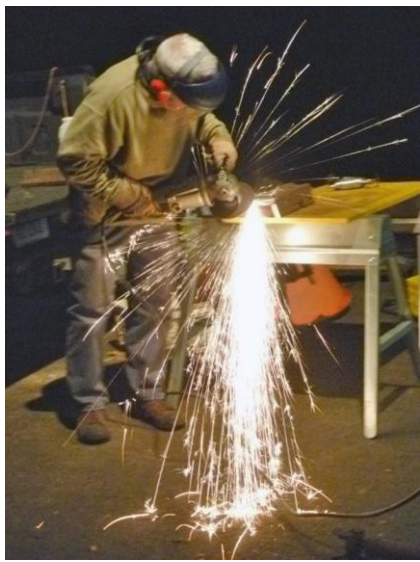
Bob Hassett grinds material in preparation of making custom-made rail joint bars for use at the museum. (C. Stanich Photo)
