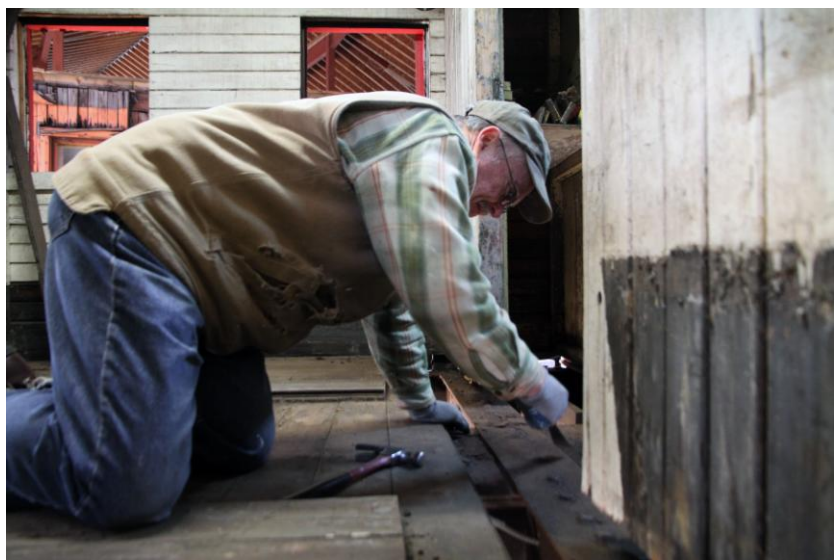
This photo taken through one of the openings of the CV #4052 caboose shows Duke York scraping rust and debris from the metal frame in the floor where rotted wood was removed. (Robert A. LaMay Photo)
