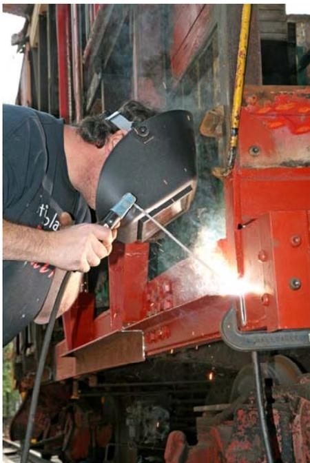
Bill Voorvaart welds a structural piece to the frame of the Central Vermont No. 4052 caboose. (LaMay Photo)
