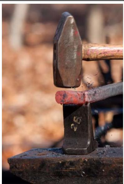
In the previous photo by Tom Nanos, a blacksmiths hammer is about to come down on a piece of molten steel. The blacksmith (better known as a smithy) forms various tools by bending and manipulating the hot steel.
