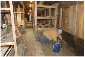
This photo shows Adrian Atkins repairing a section of floor inside coach. Note the conduit rack on the left from Bob Hassett. Getting all the materials out of the roundhouse will make it easier to move about and see displays in the roundhouse. (Robert A. LaMay Photo)
